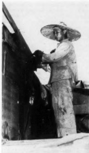
Photo by MSgt. Fred Braitach, Jr. Reluctant to survey their LVT, maintenance welds on new plate
